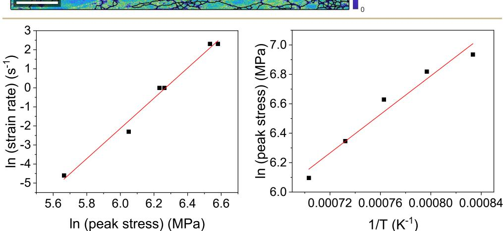
Plots showing the relationships used for calculation of parameters m (left) and r (right) needed for calculation of activation energy, Q, based on flow stress curves for alloy 680.
