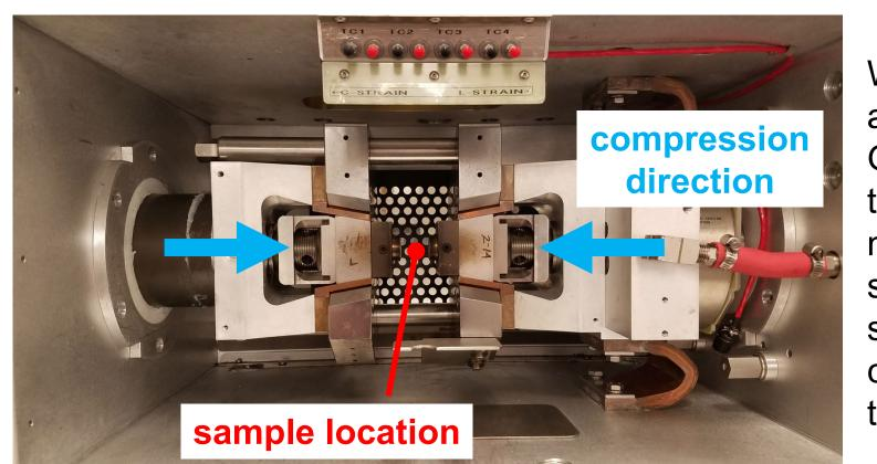
Working action of the Gleeble 3800 thermomechanical simulator, as set up for hot compression testing [1].
