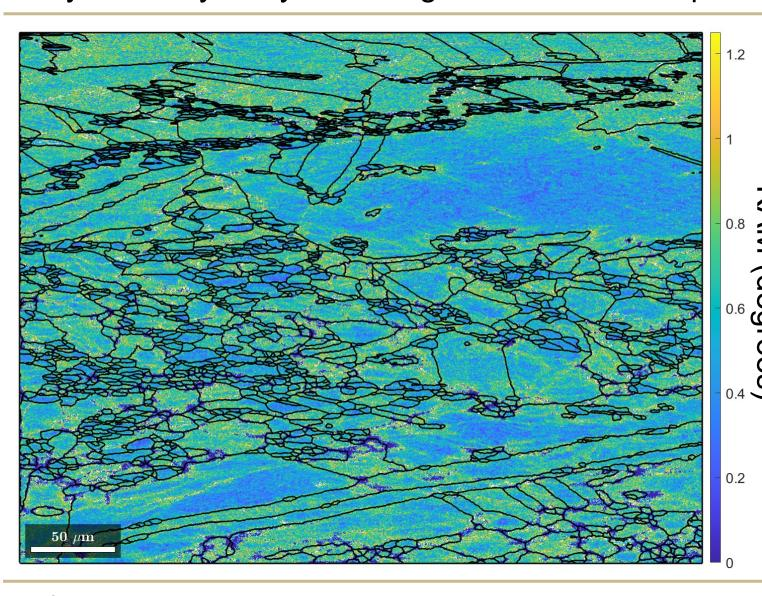
EBSD-based kernel average misorientation (KAM) map of sample A on JMAK curve. Small recrystallized grains with low internal misorientation can bee seen in dark blue.
